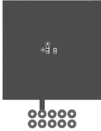
a. 350^\circ\text{C/W} when mounted on a 1\text{ in}^2 pad of 2 oz copper.
